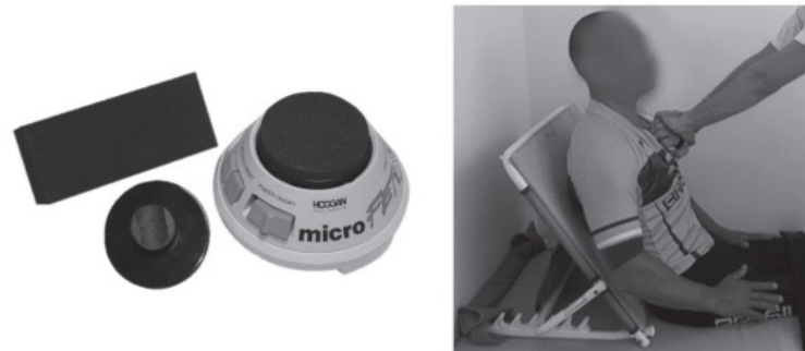
Figure 3 – Left: Device used to measure trunk flexion strength (Handheld dynamometer). Right: Athlete position while performing trunk flexion strength test.
